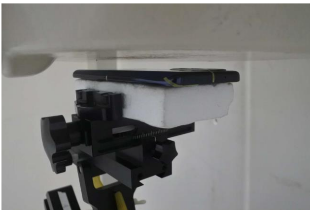
Back, Test Separation 12 mm
