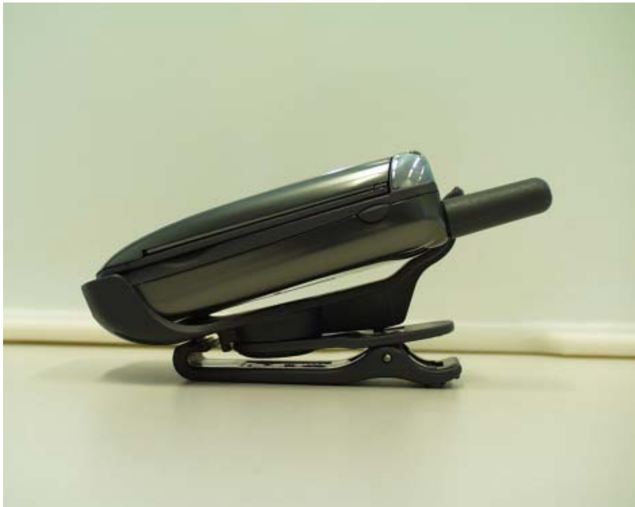
Figure 9. Separation Distance of 33 mm from Tip of Antenna to Flat Phantom and 10 mm from the bottom of the clip when rotated 0°.
