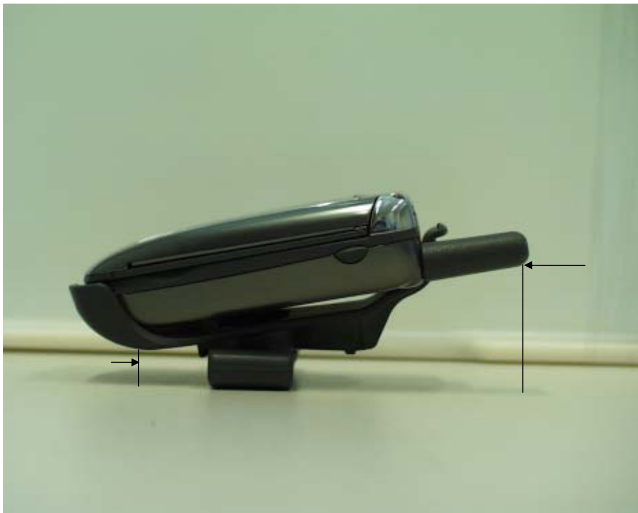
Figure 8. Separation Distance of 25 mm from Tip of Antenna to Flat Phantom and 8 mm from the bottom of the clip when rotated +90° (Clockwise Direction)
