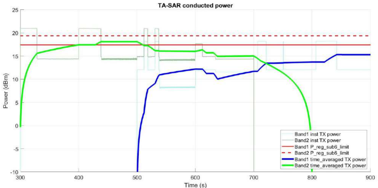
Figure 6- 46 Time-averaged conducted TX power over time
