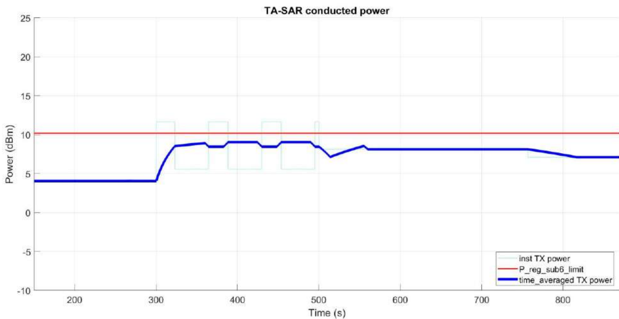
Figure 6- 22 Time-averaged conducted TX power over time
