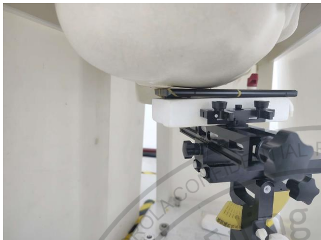
Right Cheek, Test Separation 0 mm
