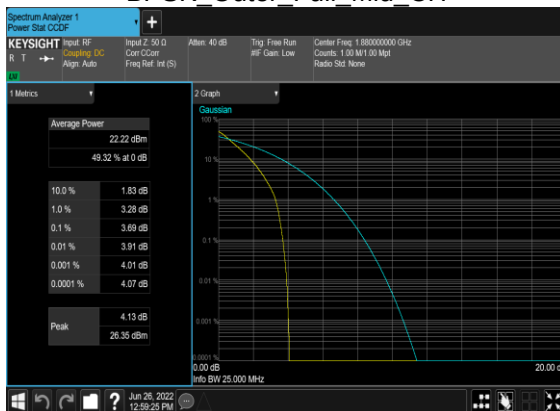
B7_N2(20M)_DFT-s-OFDM_PI_2-BPSK Outer Full Mid CH
