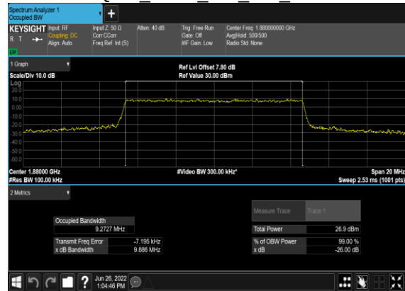
B7_N2(10M)_CP-OFDM_16 QAM Outer Full Mid CH
