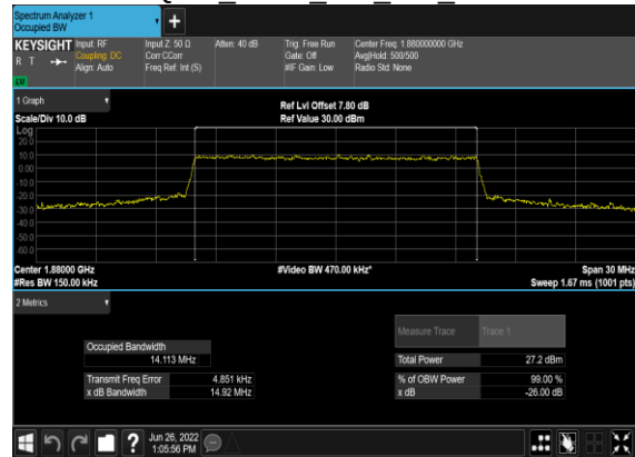
B7_N2(15M)_CP-OFDM_16 QAM Outer Full Mid CH
