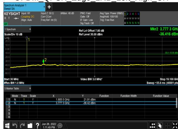
B7_N2(5M)_DFT-s-OFDM QPSK Edge 1RB Left High CH
