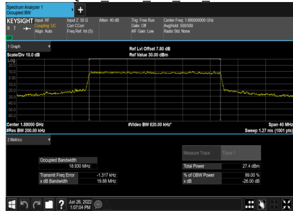
B7_N2(20M)_CP-OFDM_16 QAM Outer Full Mid CH
