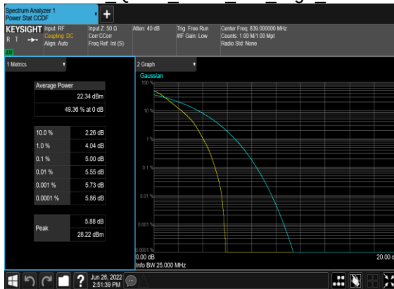
B7_N5(20M)_DFT-s-OFDM QPSK Outer Full High CH
