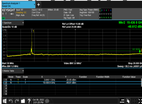
N48(100M)_DFT-s-OFDM QPSK Edge 1RB Right Low CH
