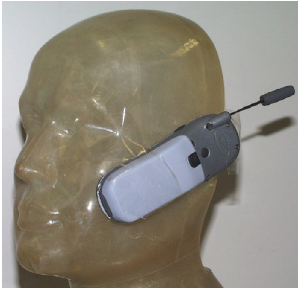
Figure 8. Phone with Antenna Extended against Phantom Head
