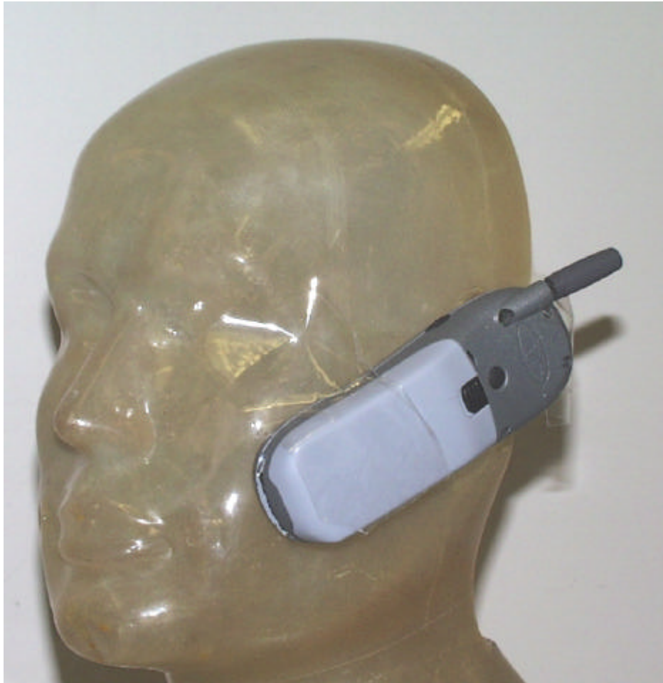
Figure 7. Phone with Antenna Retracted against Phantom Head
