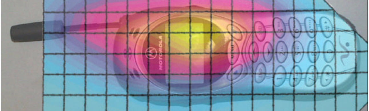
Figure 1. Typical 800 Analog Contour Plot Overlaid on Face of Phone.
