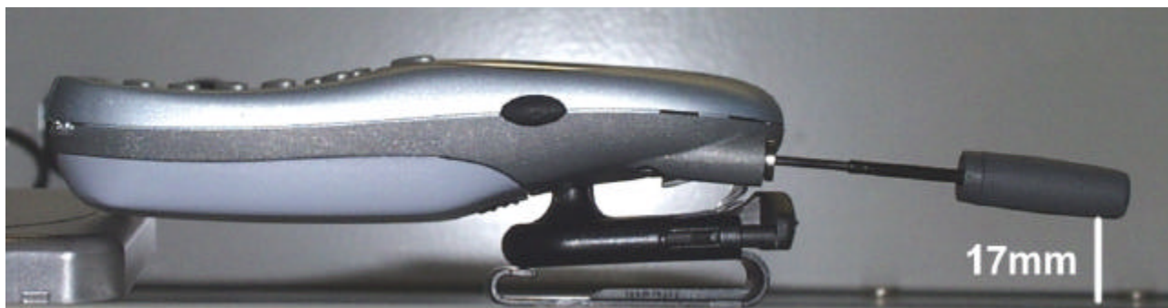
Figure 11. Distance Provided from Belt Clip with Antenna Extended.
