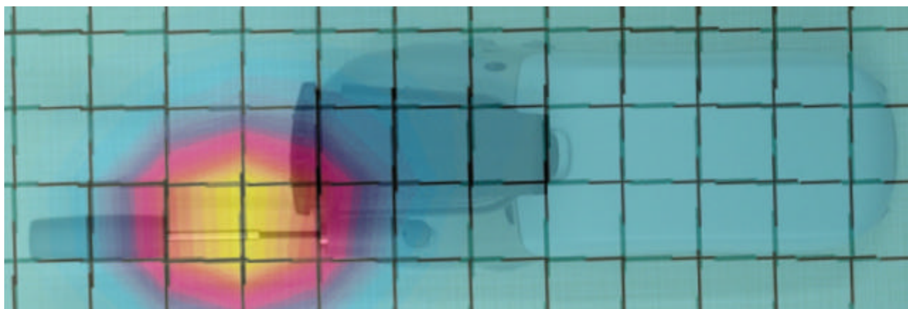
Figure 5. Typical 1900 CDMA Body Worn Contour Plot Overlaid on Back of Phone.
