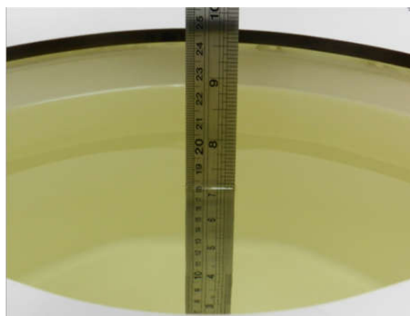
Fig 11.2 Photo of Liquid Height for Body SAR
