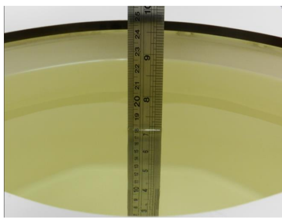
Fig 11.2 Photo of Liquid Height for Body SAR
