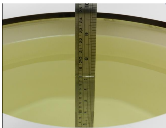
Fig 11.2 Photo of Liquid Height for Body SAR
