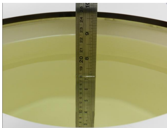
Fig 11.2 Photo of Liquid Height for Body SAR
