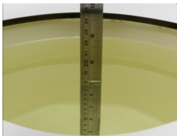
Fig 11.2 Photo of Liquid Height for Body SAR
