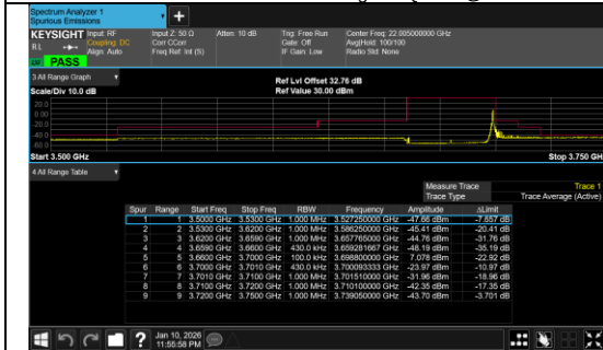
Conducted Band Edge CHP Range9 PASS Band 48 40MHz/3679.98/High QPSK 100@0
