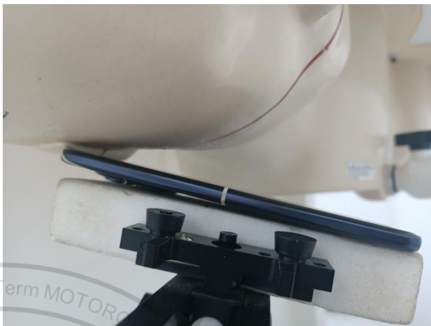
Right Tilted, Test Separation 0 mm
