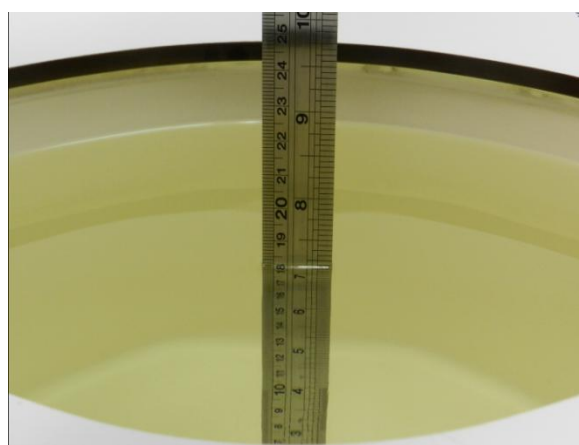
Fig 11.2 Photo of Liquid Height for Body SAR
