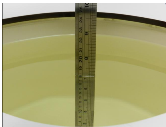
Fig 11.2 Photo of Liquid Height for Body SAR
