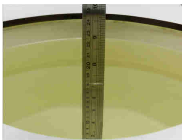
Fig 11.2 Photo of Liquid Height for Body SAR
