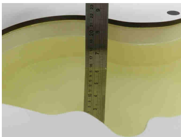
Fig 11.1 Photo of Liquid Height for Head SAR
