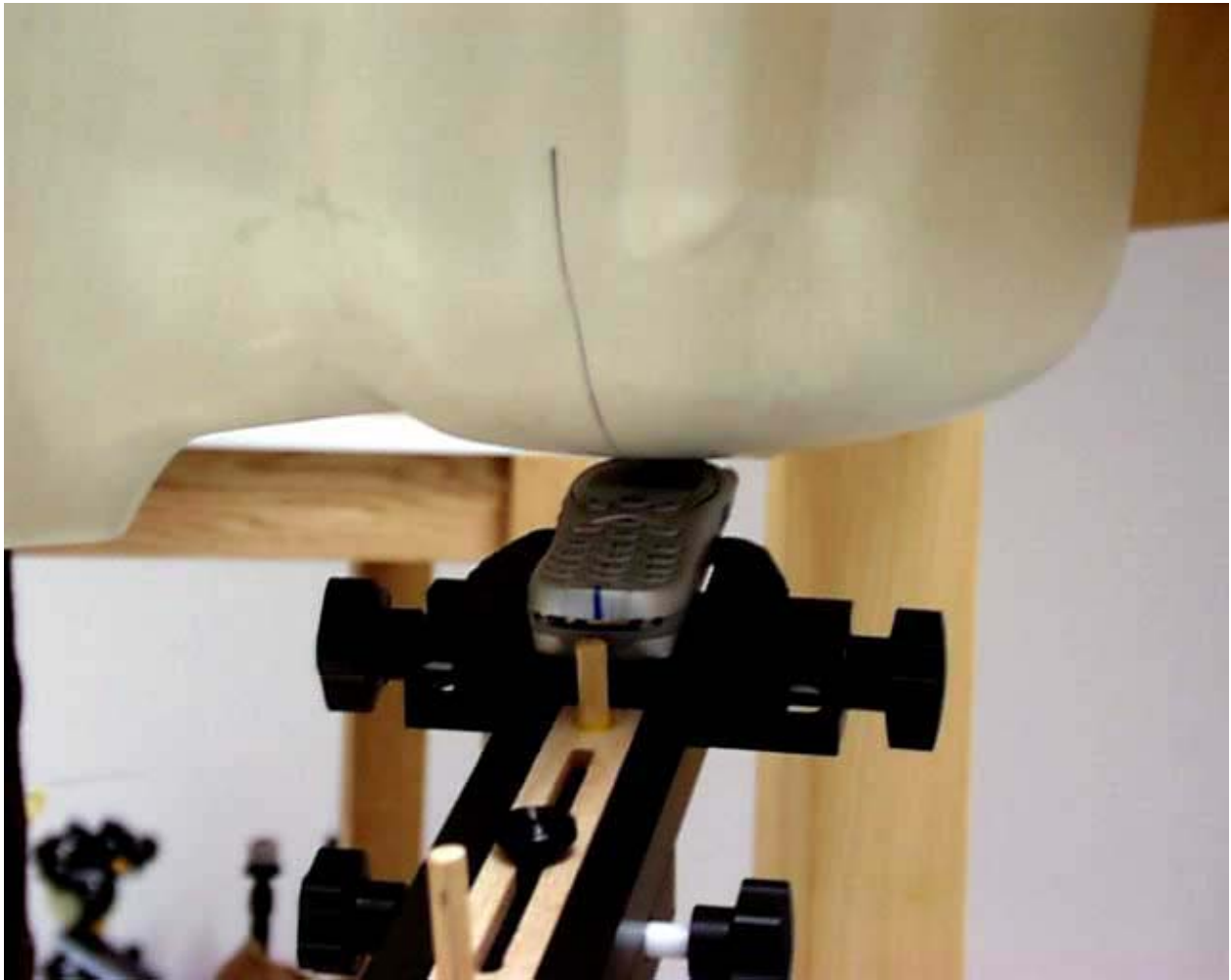
Figure 16. Bottom of Phone Seen in 15 Degree Tilt Testing Configuration
