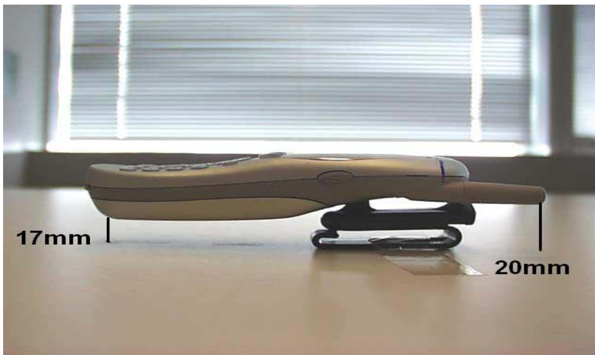
Figure 10. Separation Distance Provided from Plastic Belt Clip
