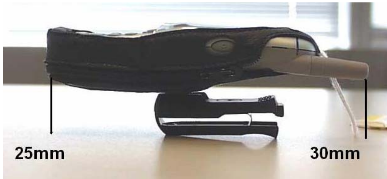
Figure 9. Distance of the Antenna (Fixed) to the Base of the Flat Phantom
