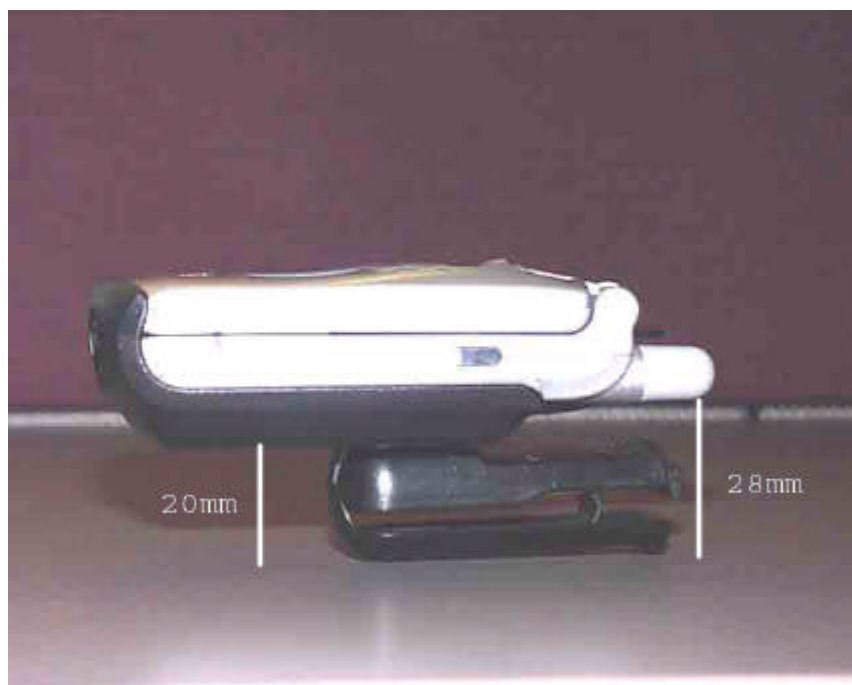
Figure 16. Phone in Accessory Against Flat Phantom with Head Set Attached
