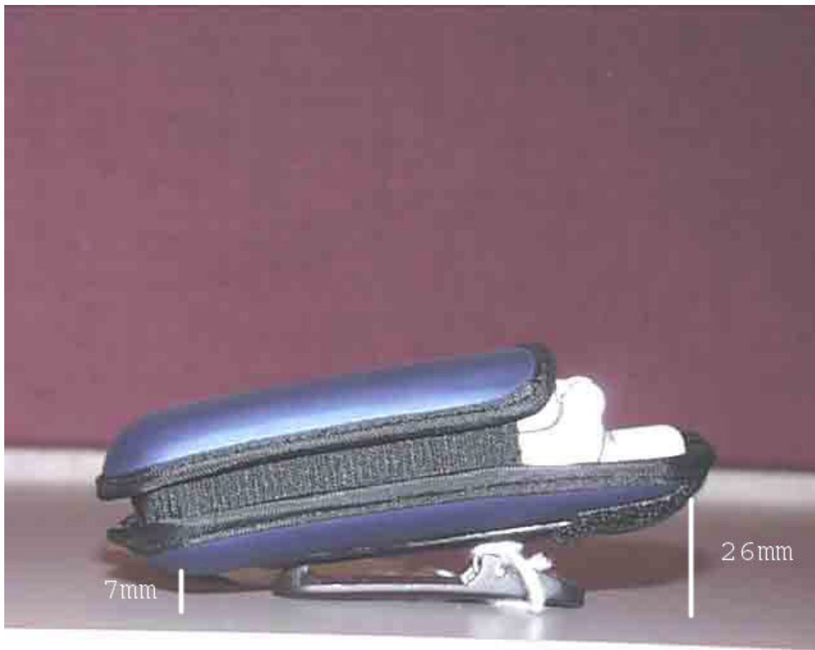
Figure 15. Phone in Navy Pouch Showing Separation Distance
