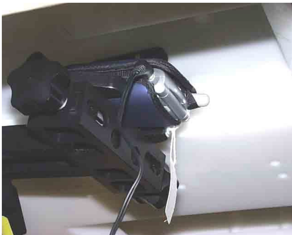
Figure 16. Phone in Accessory Against Flat Phantom with Head Set Attached
