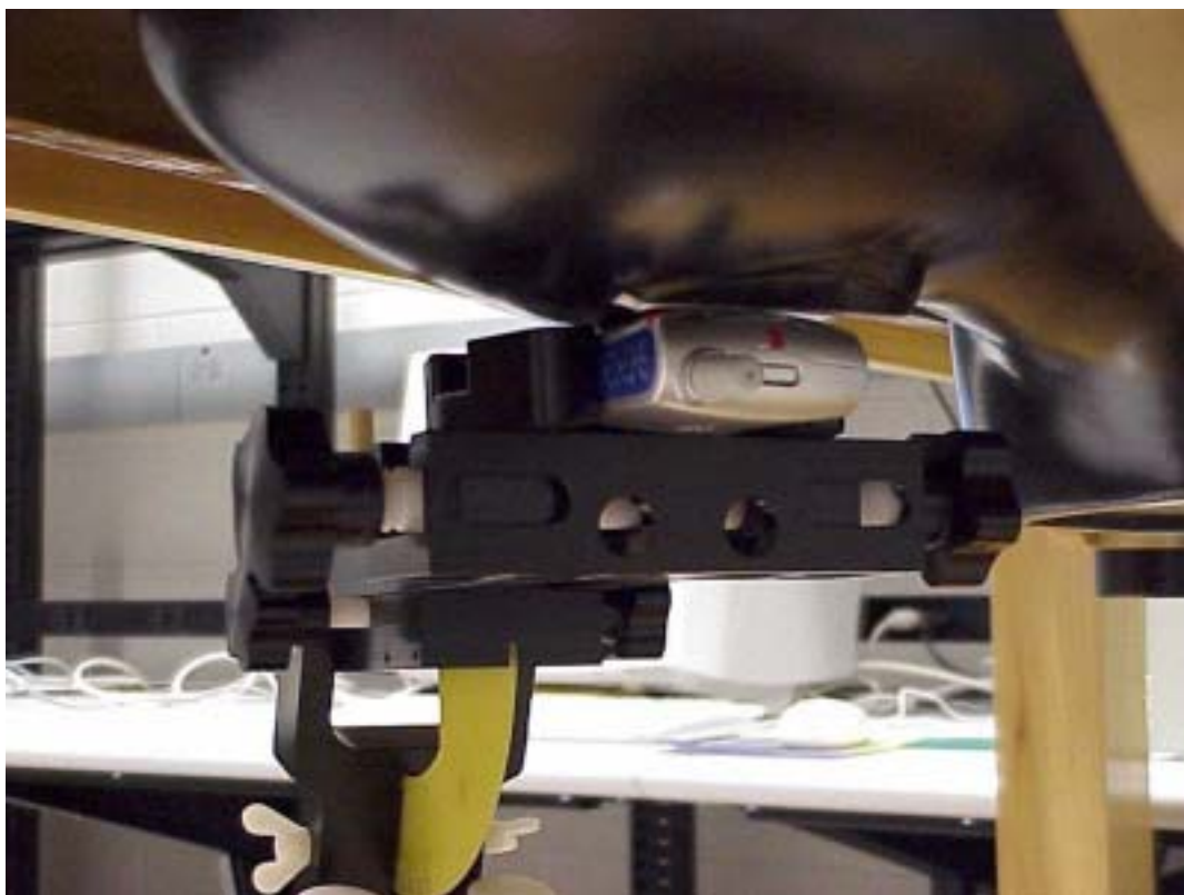
Figure 13. Back View of Phone Placed Against Head with Antenna Fixed
