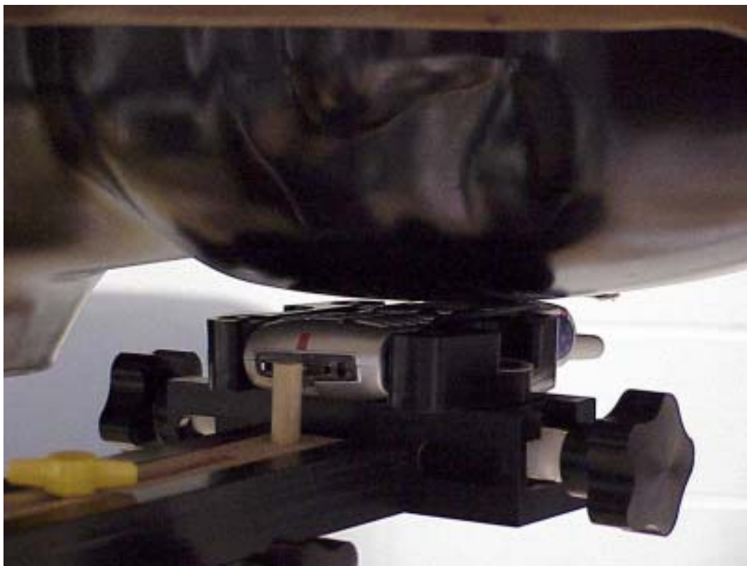
Figure 12. Front View of Phone Placed Against Head with Antenna Fixed
