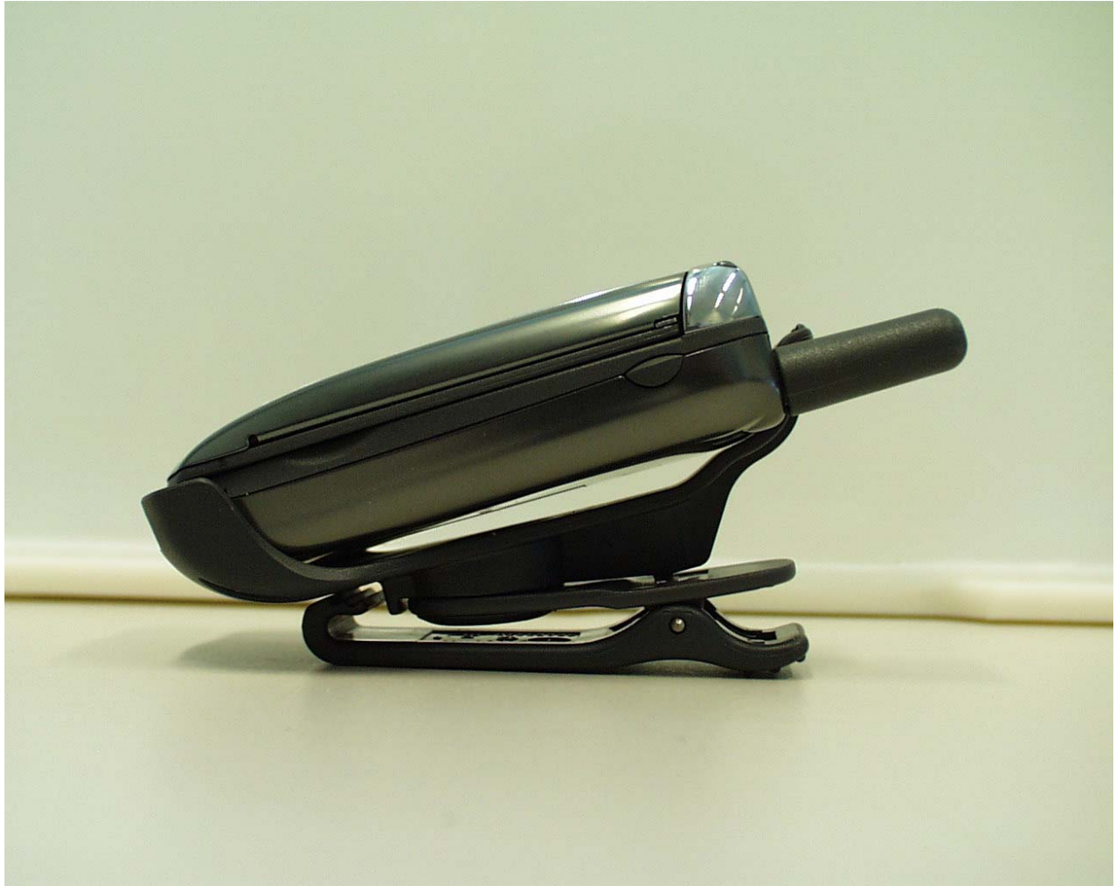
Figure 12. Separation Distance from Tip of Antenna to Flat Phantom when rotated 0°
