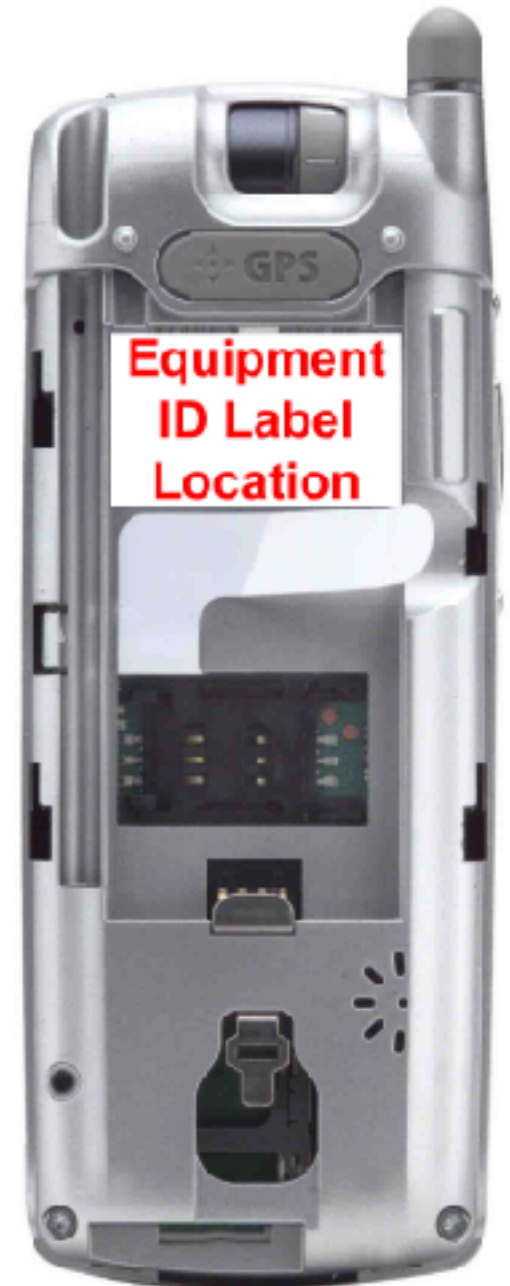
Rear View Showing ID Label
