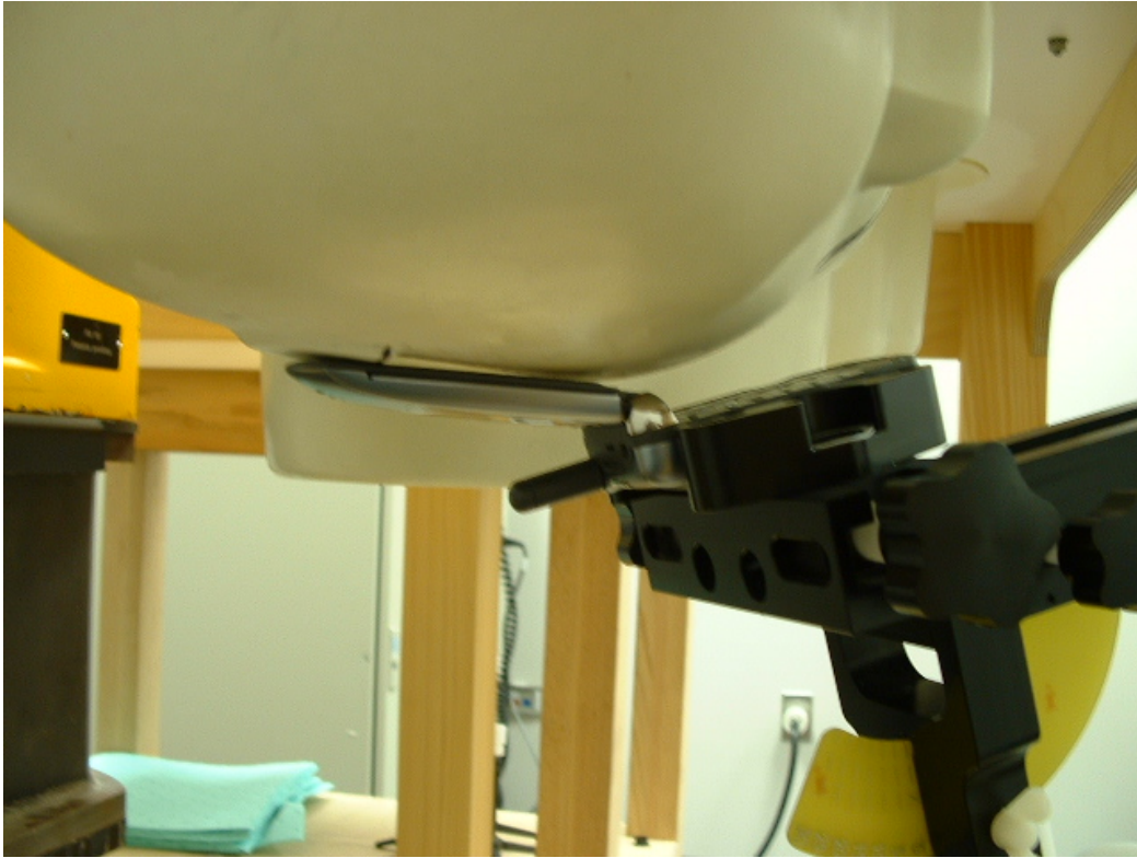
Figure 5. Phone against the head (Cheek Touch)
