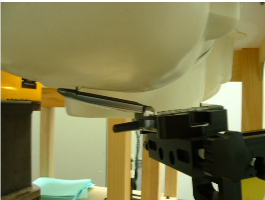
Figure 6. Phone against the head (15° Tilt)
