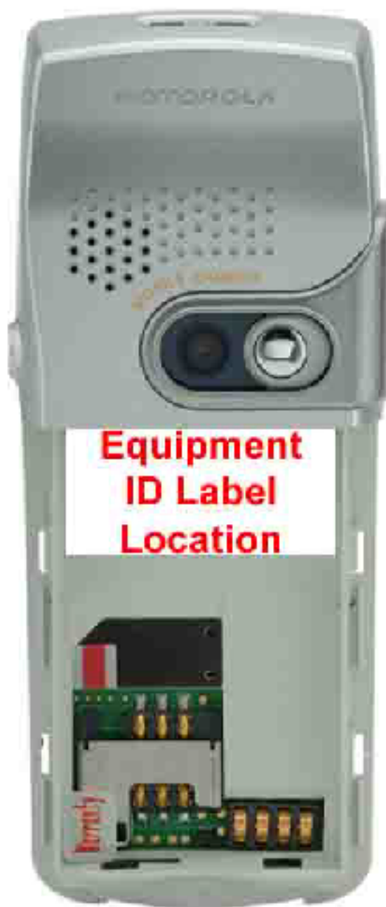
Rear View with Battery Removed to Show Equipment ID Label
