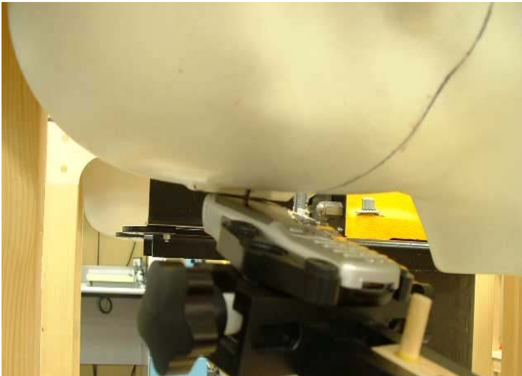
Figure 12. Phone against the head (15° tilt)
