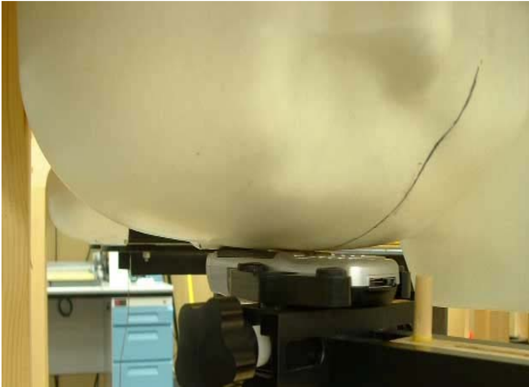
Figure 11. Phone against the head (Cheek Touch)
