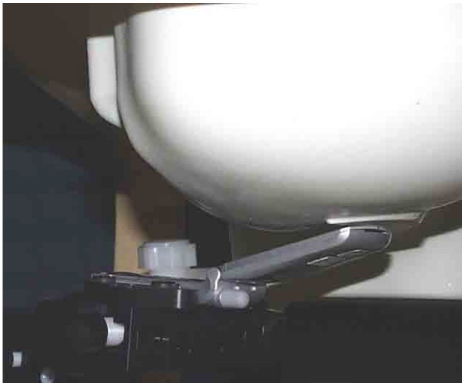
Figure 15. Phone Against the Head Phantom (Back View – 15° Tilt)
