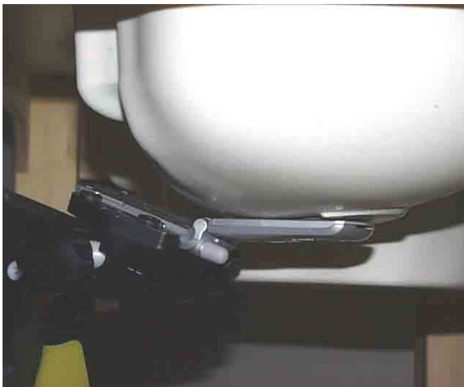
Figure 13. Phone Against the Head Phantom (Back View – Cheek Touch)
