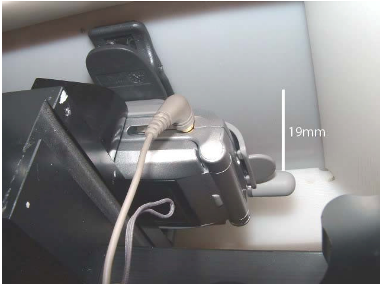
Figure 11. Phone with Holster Against the Flat Phantom
