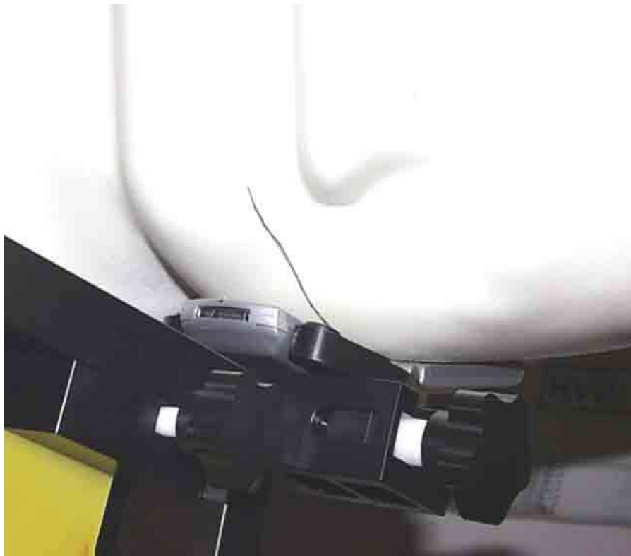
Figure 12. Phone Against the Head Phantom (Front View - Cheek Touch)
