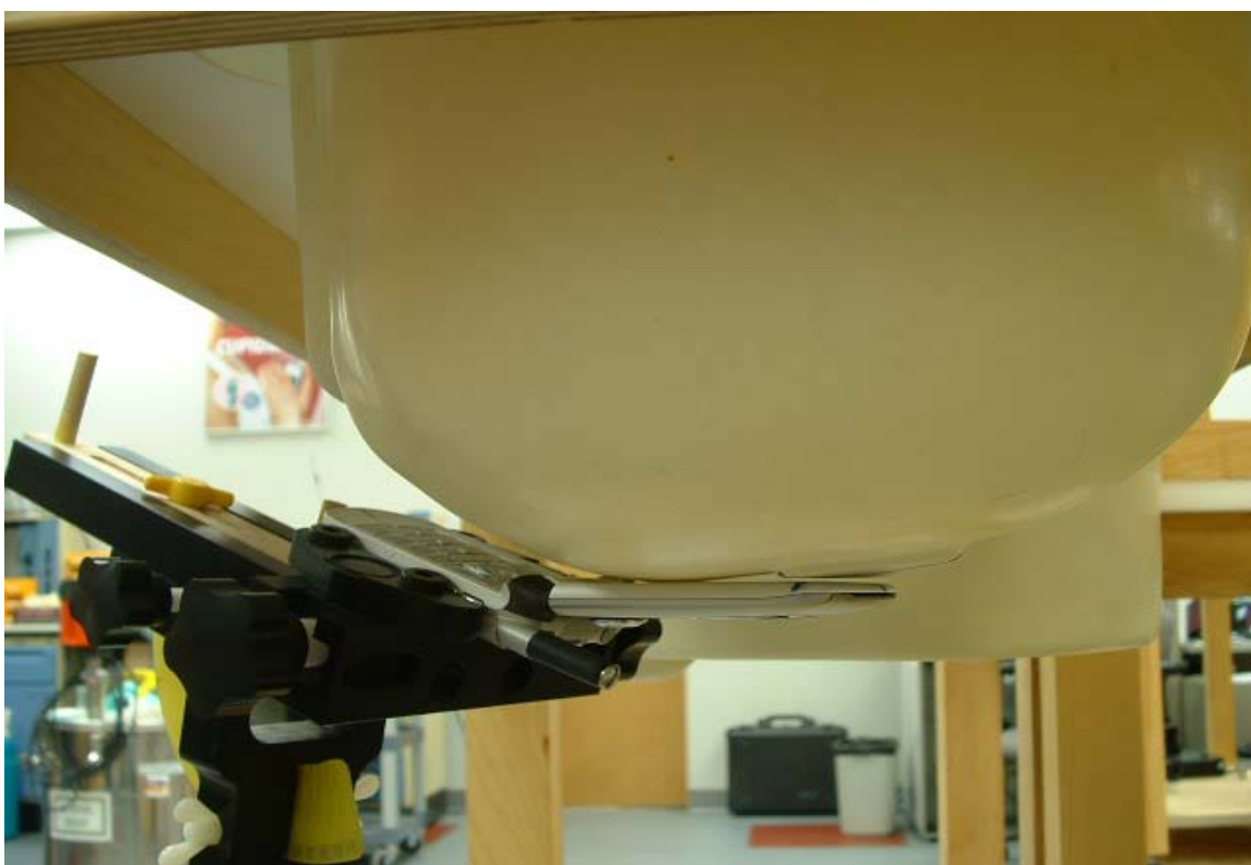
Figure 15. Phone Against the Head with Antenna Retracted (Back View – Cheek Touch)
