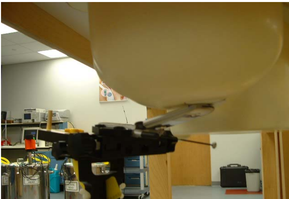
Figure 21. Phone Against the Head with Antenna Extended (Back View – 15°Tilt)
