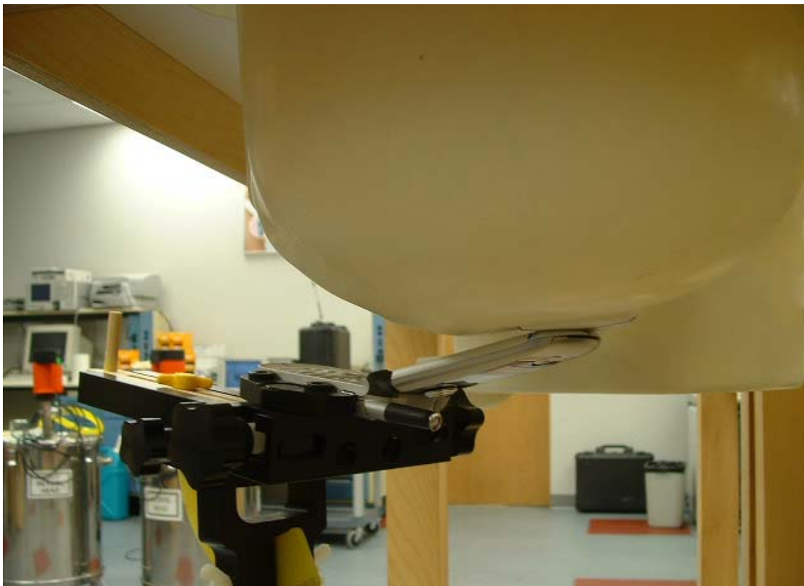
Figure 19. Phone Against the Head with Antenna Retracted (Back View – 15°Tilt)
