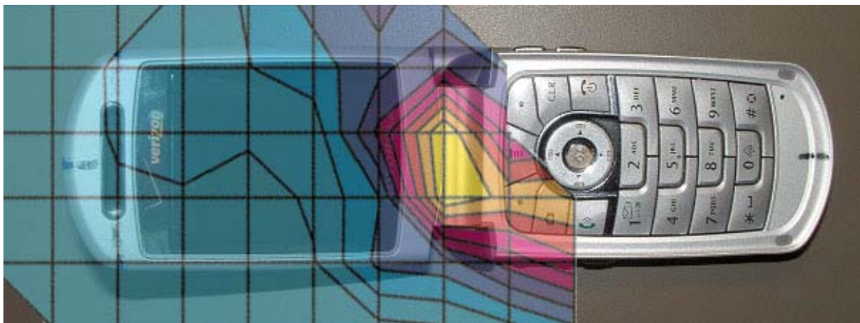
Figure 4. Typical 1900MHz Head Adjacent Contour Overlaid on Phone with Antenna Retracted (Cheek Touch)
