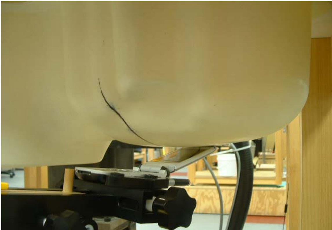
Figure 18. Phone Against the Head with Antenna Retracted (Front View – 15°Tilt)
