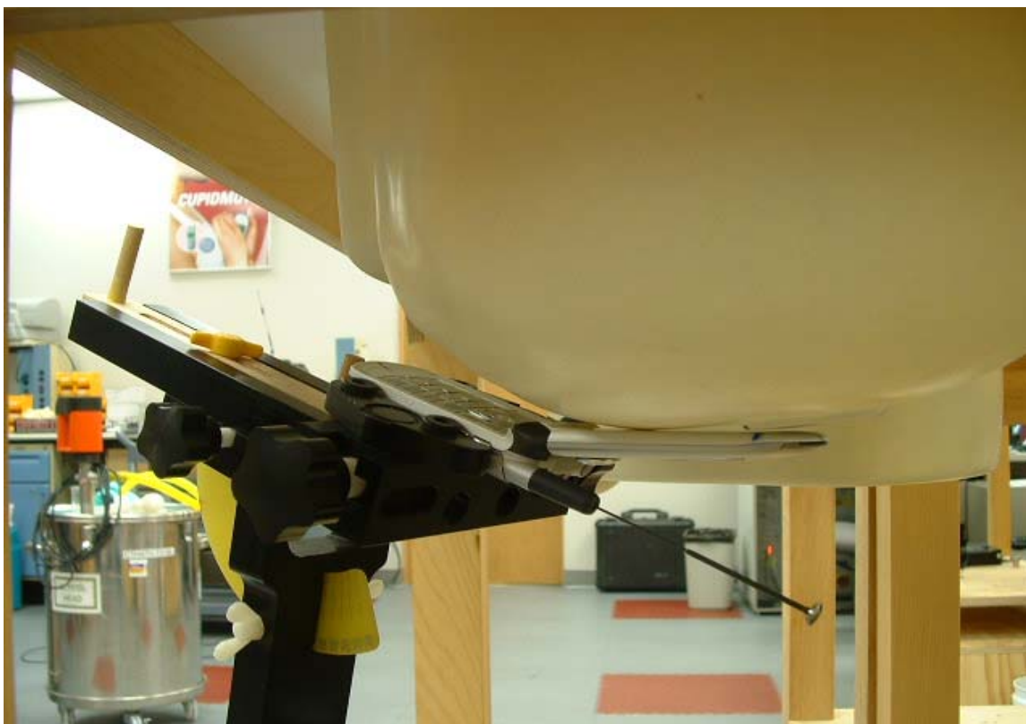
Figure 17. Phone Against the Head with Antenna Extended (Back View – Cheek Touch)
