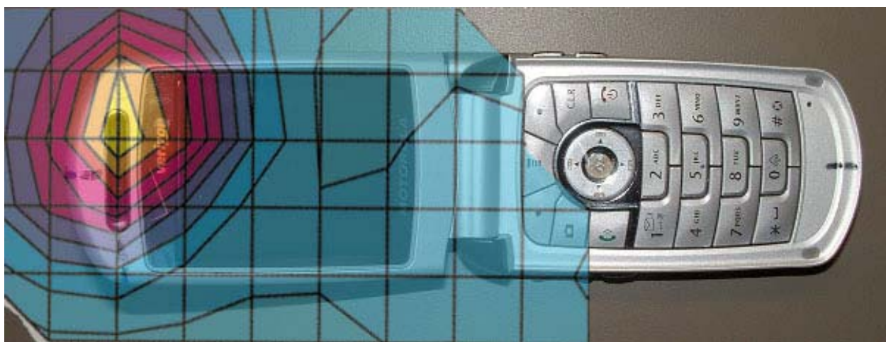
Figure 6. Typical 1900MHz Head Adjacent Contour Overlaid on Phone with Antenna Extended (15 ° Tilt)
