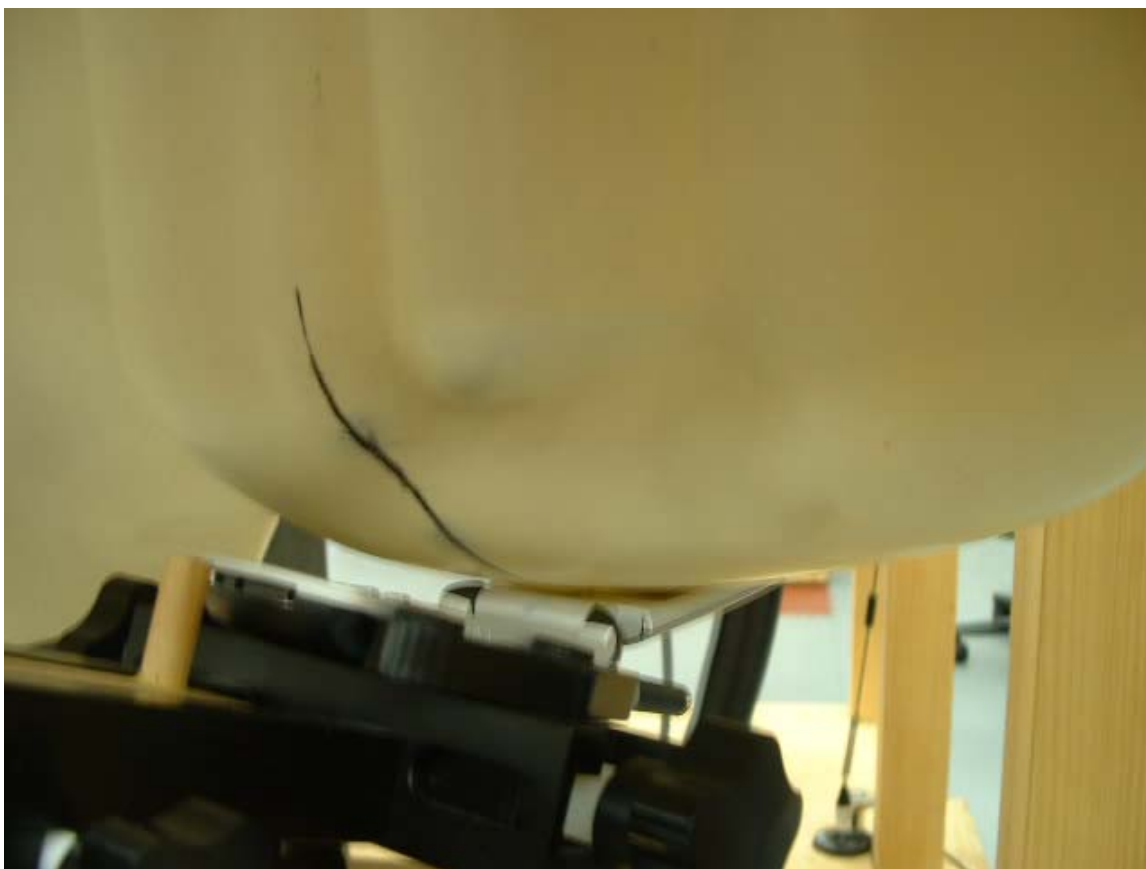
Figure 14. Phone Against the Head with Antenna Retracted (Front View – Cheek Touch)
