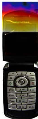
Figure 28 Sample H-field Scan Overlay
