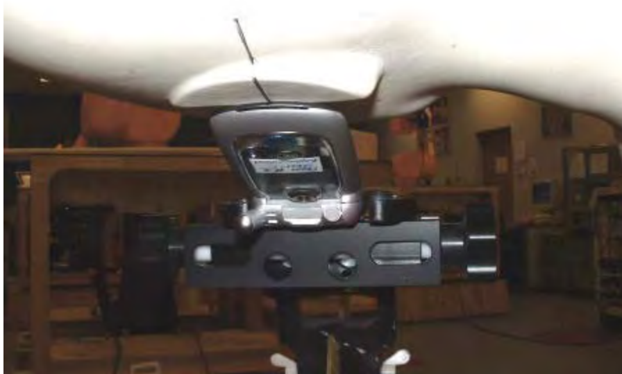
Figure 32. Phone Against the Head with Antenna Retracted (Back View – 15°Tilt)
