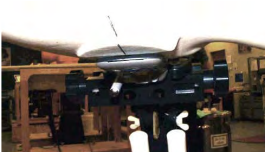
Figure 28. Phone Against the Head with Antenna Retracted (Back View – Cheek Touch)
