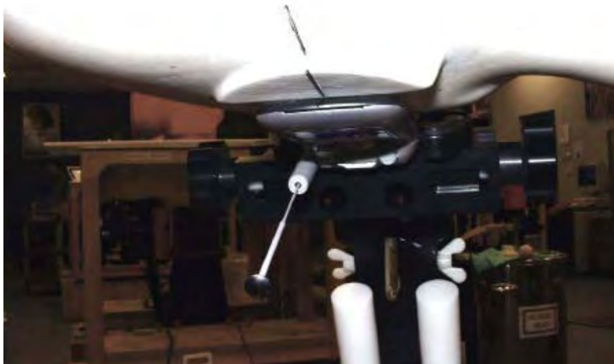
Figure 30. Phone Against the Head with Antenna Extended (Back View – Cheek Touch)
