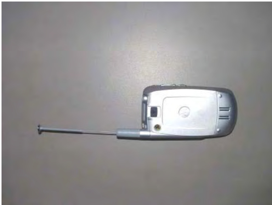
Figure 16.Back of Phone with Antenna Extended
