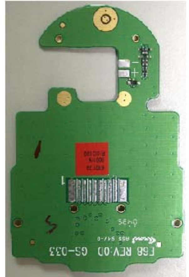
Sub Board Display Removed
