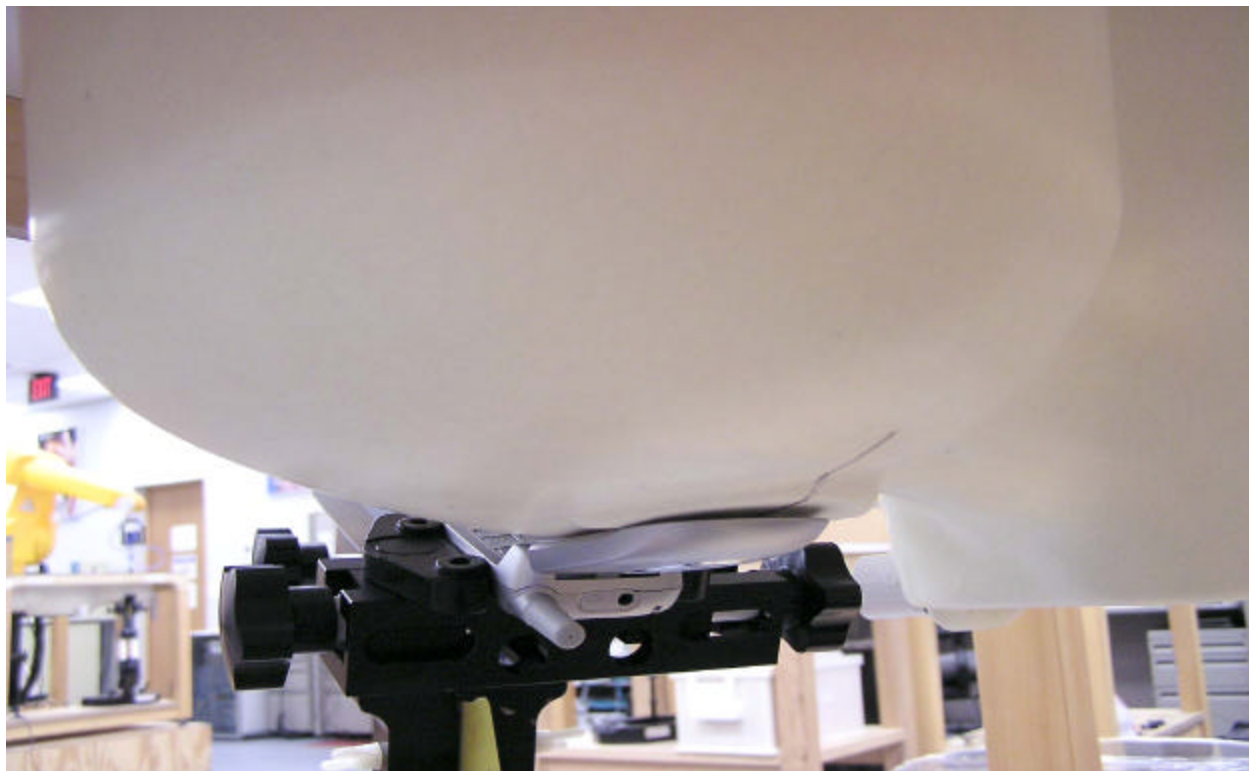
Figure 12. Phone Against the Head Phantom (Back View – Cheek Touch)
