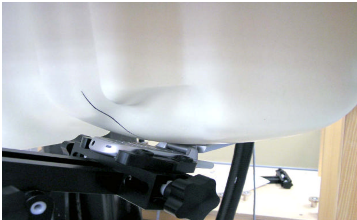
Figure 11. Phone Against the Head Phantom (Front View - Cheek Touch)
