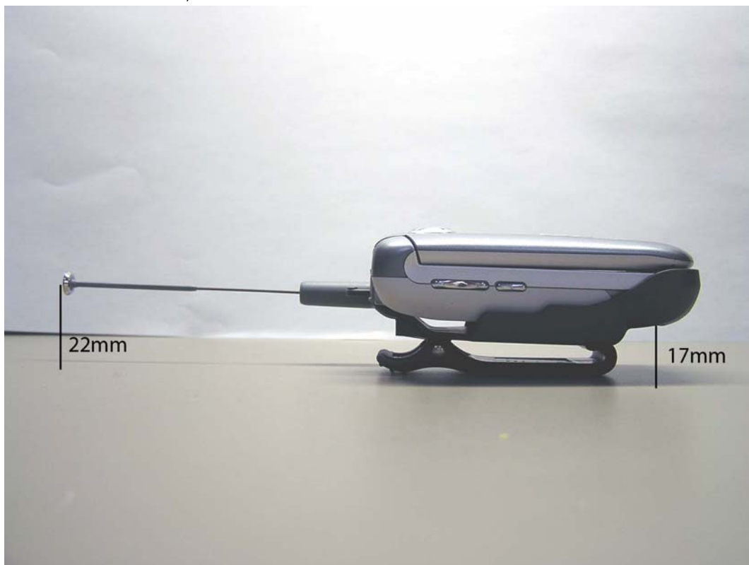
Figure 9.Side of Phone in Holster with Antenna Extended and Standard Battery cover
