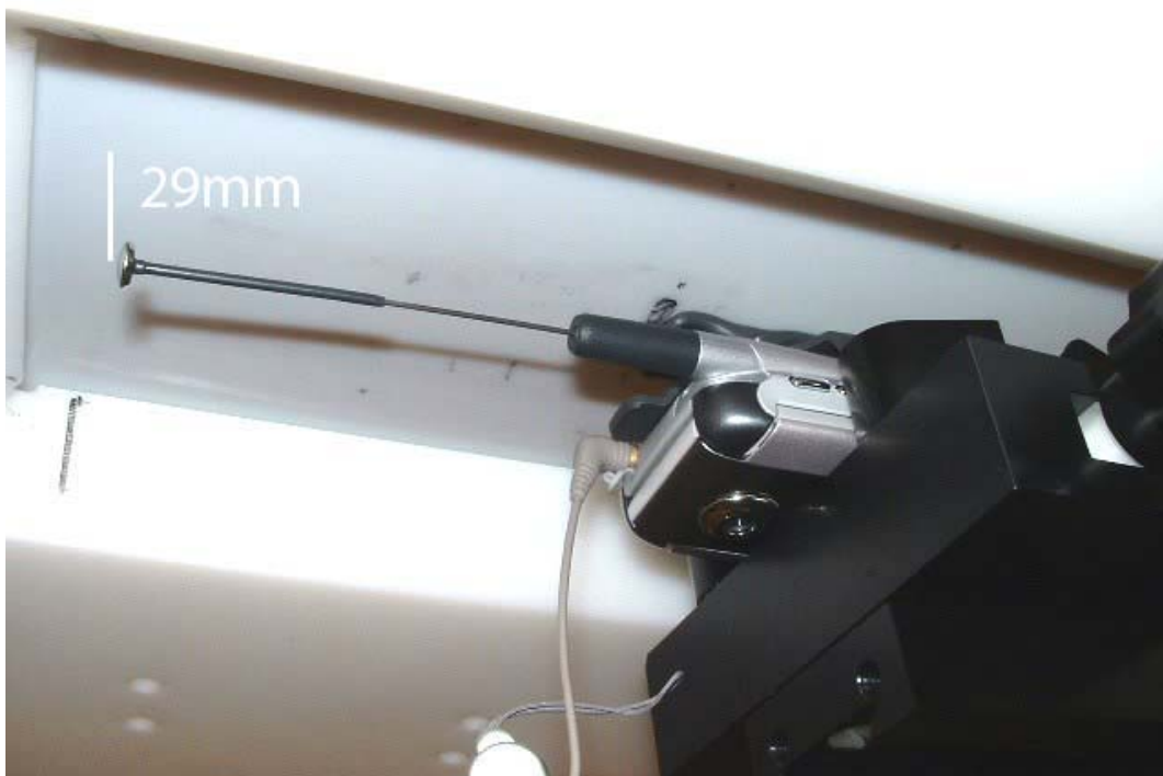
Figure 21. Phone in Holster Against the Flat Phantom with Antenna Extended
