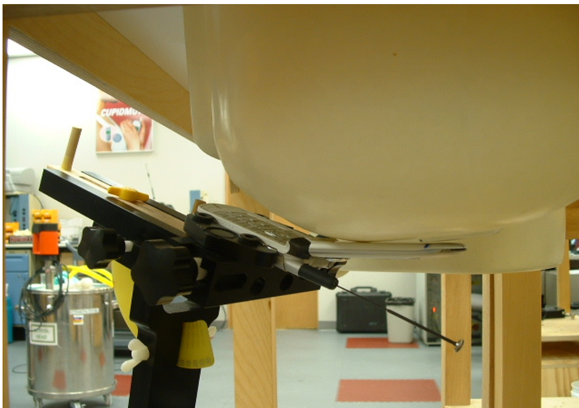
Figure 15. Phone Against the Head with Antenna Extended (Back View – Cheek Touch)
