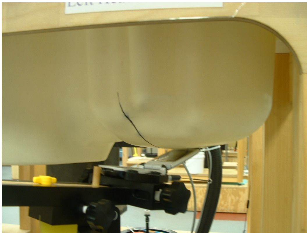
Figure 18. Phone Against the Head with Antenna Extended (Front View – 15°Tilt)
