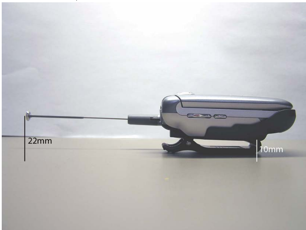
Figure 11. Side of Phone in Holster with Antenna Extended and Extended Battery cover
