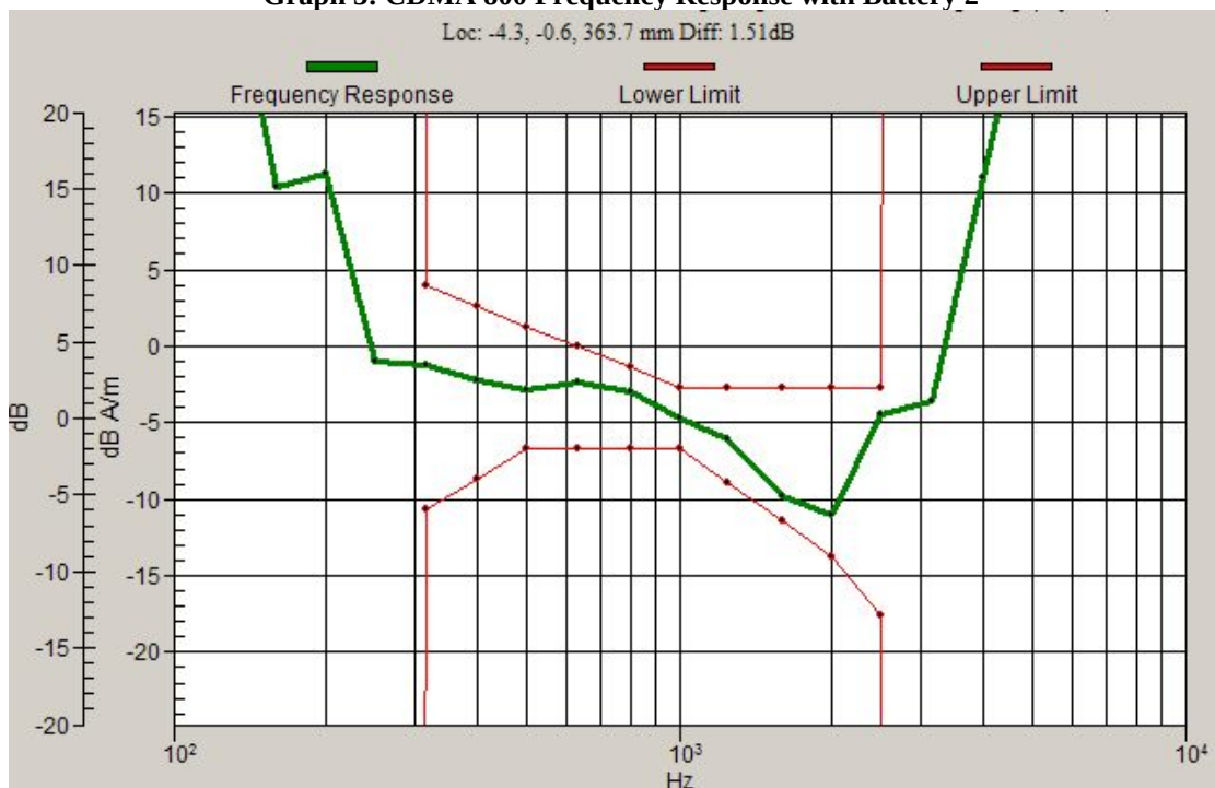
Graph 3: CDMA 800 Frequency Response with Battery 2
