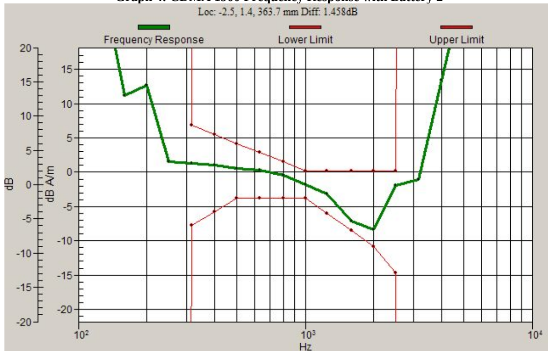
Graph 4: CDMA 1900 Frequency Response with Battery 2
