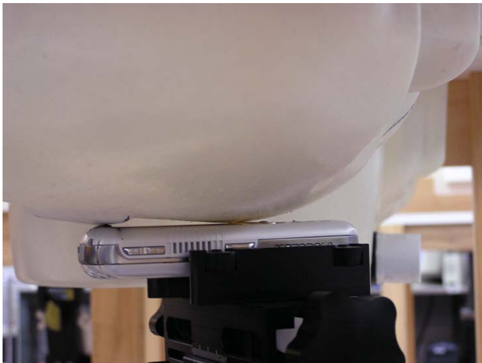
Figure 3. Phone Against the Head Phantom (Cheek Touch)
