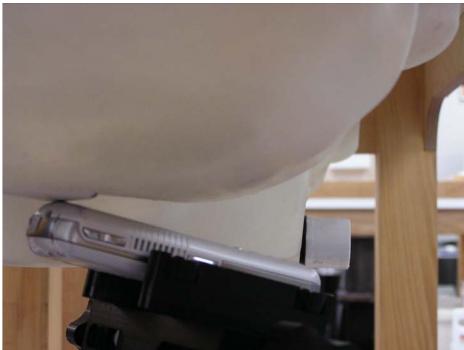
Figure 4. Phone Against the Head Phantom (15°Tilt)
