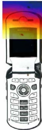
Figure 28 Sample H-field Scan Overlay
