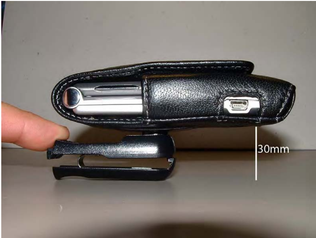
Figure 21. Side View; SYN1066A Case with SYN8763B Belt Clip
