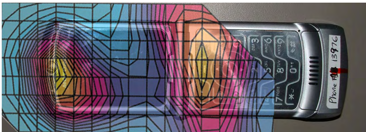
Figure 4. Typical 1900MHz GSM Head Adjacent Contour Overlaid on Phone (15 ° Tilt)
