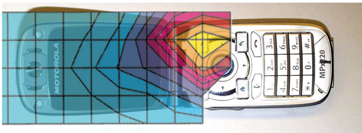
Figure 1. Typical 850MHz Head Adjacent Contour Overlaid on Phone (Cheek Touch)
