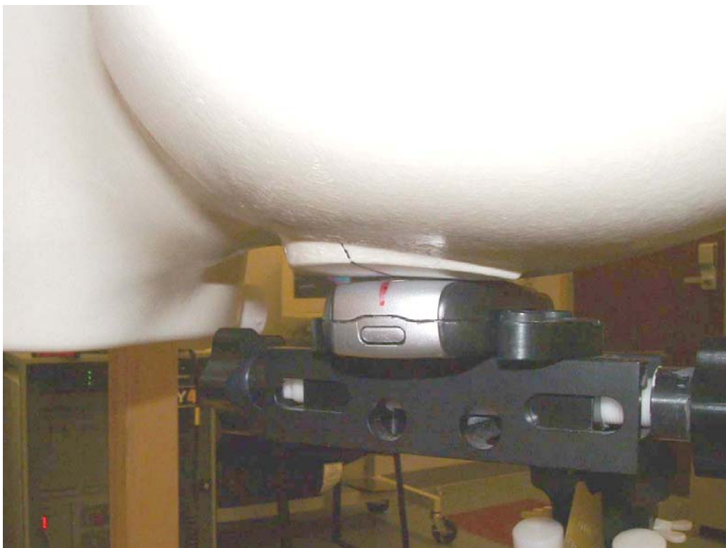
Figure 4. Phone Against the Head Phantom (Back View – Cheek Touch)
