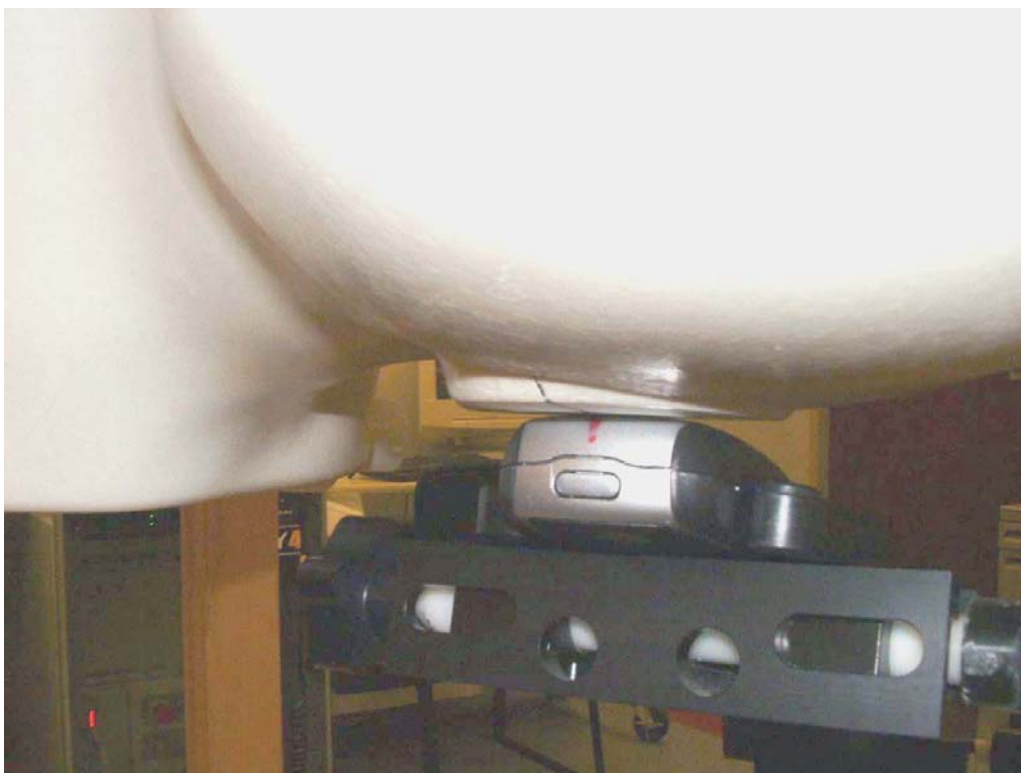
Figure 6. Phone Against the Head Phantom (Back View – 15°Tilt)
