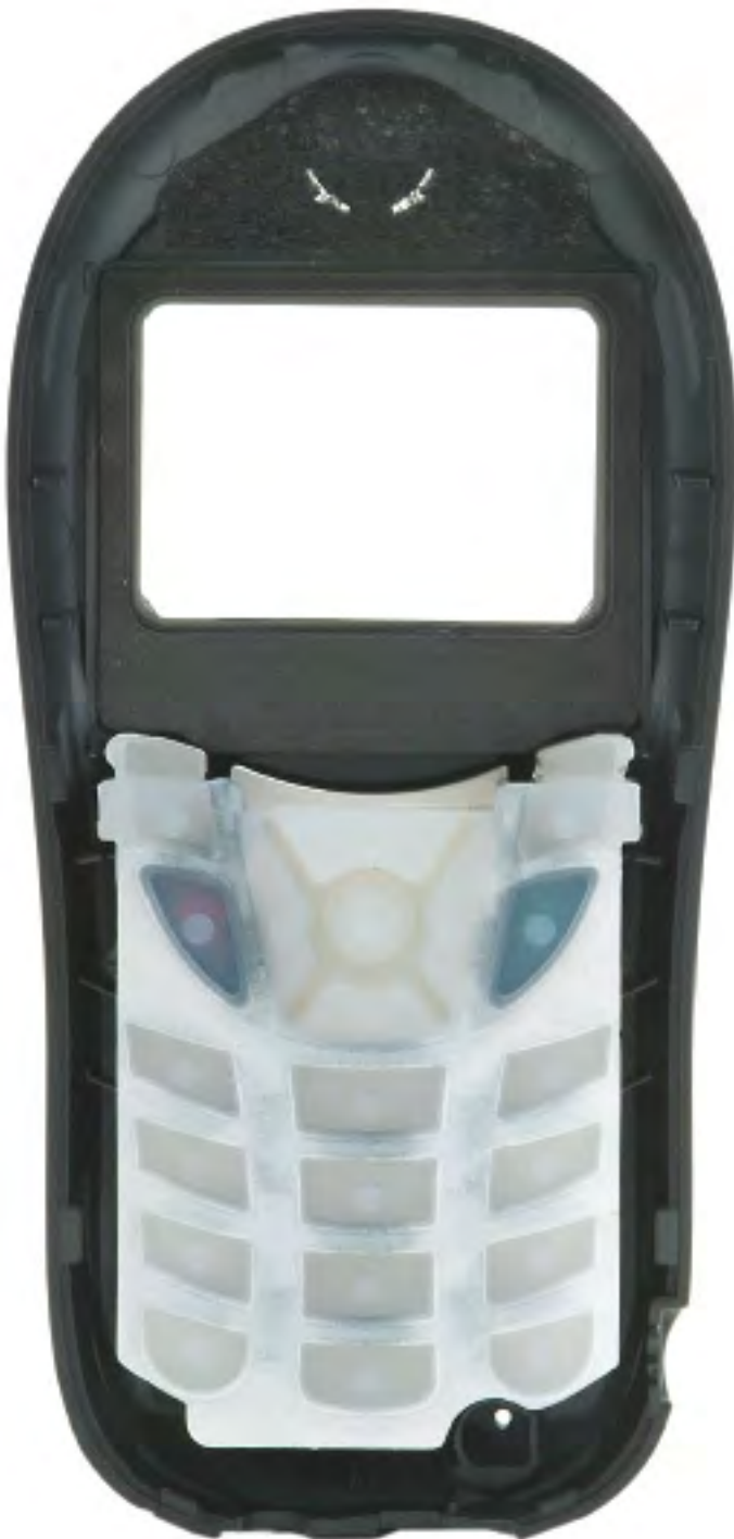
Front Housing Internal View
