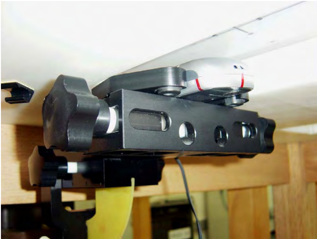
Figure 7. Phone Against the Flat Phantom
