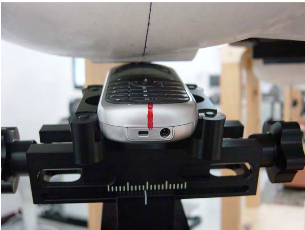
Figure 5 Phone Against the Head Phantom (Front View – 15°Tilt)
