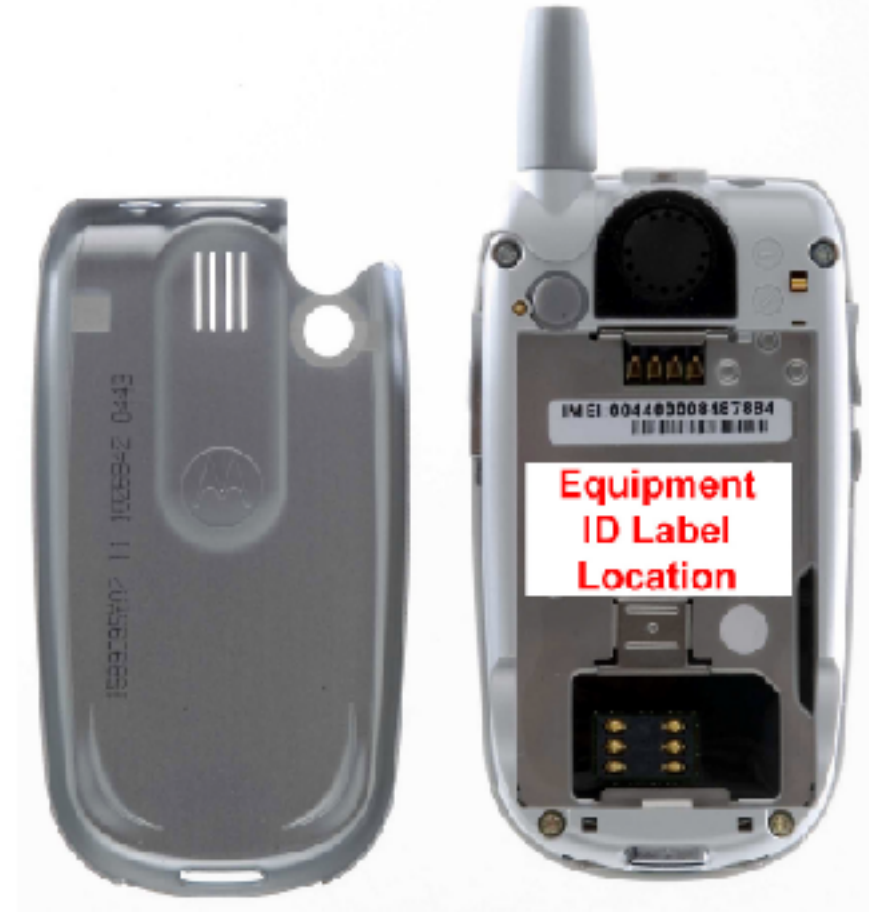
Rear View with Battery Cover Removed Showing ID Label
