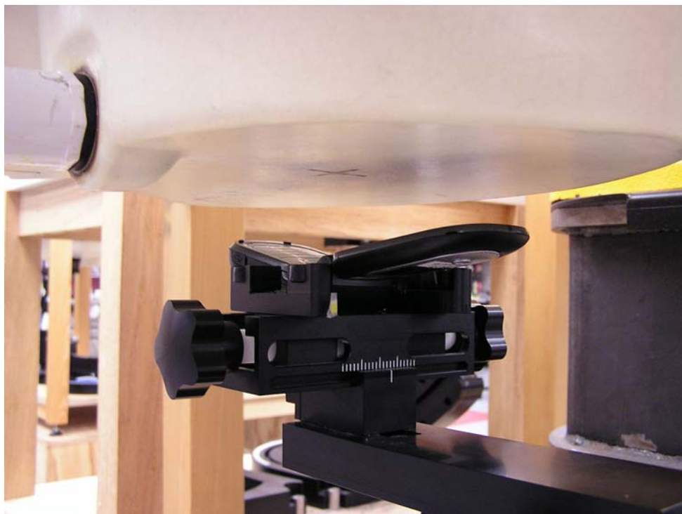
Figure 10 – Transceiver in PTT Mode, Flip Open, Front of Phone 25mm from Flat of SAM Phantom position
