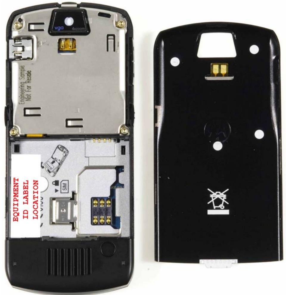
Rear View with NFC & Battery Cover Removed Showing ID Label
