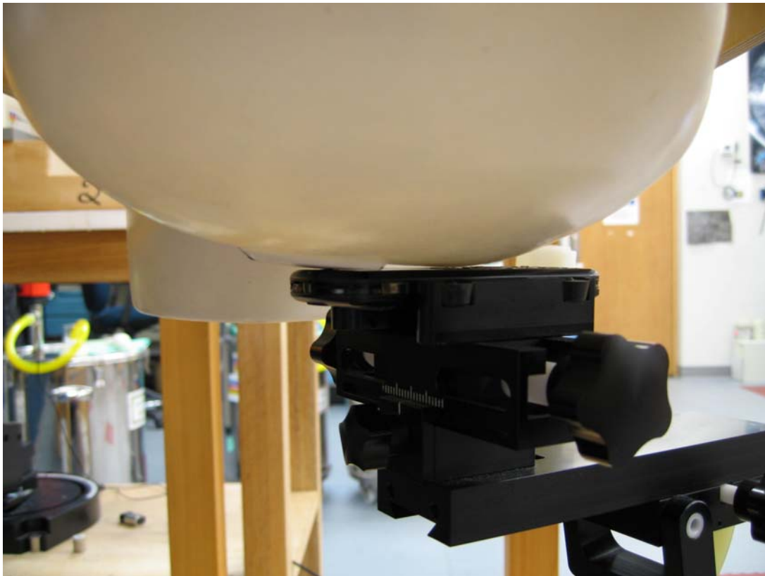
Figure 4 – Transceiver against head, Cheek Touch position
