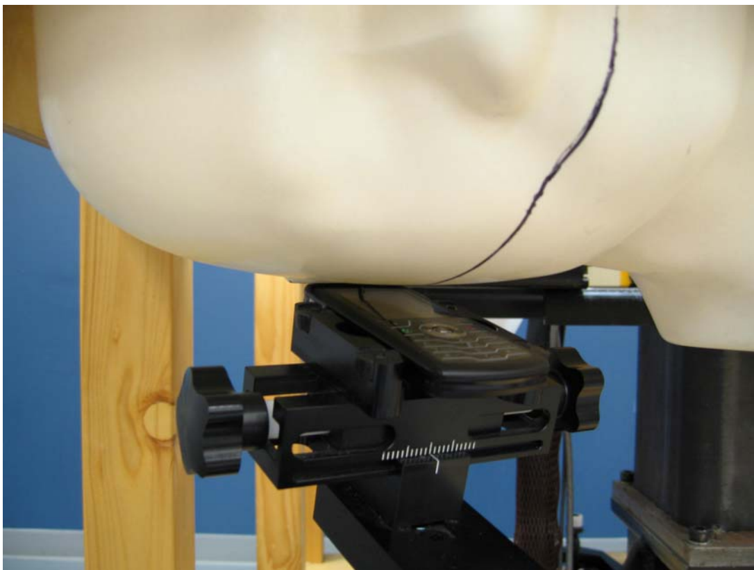
Figure 5 – Transceiver against head, 15° Tilt position
