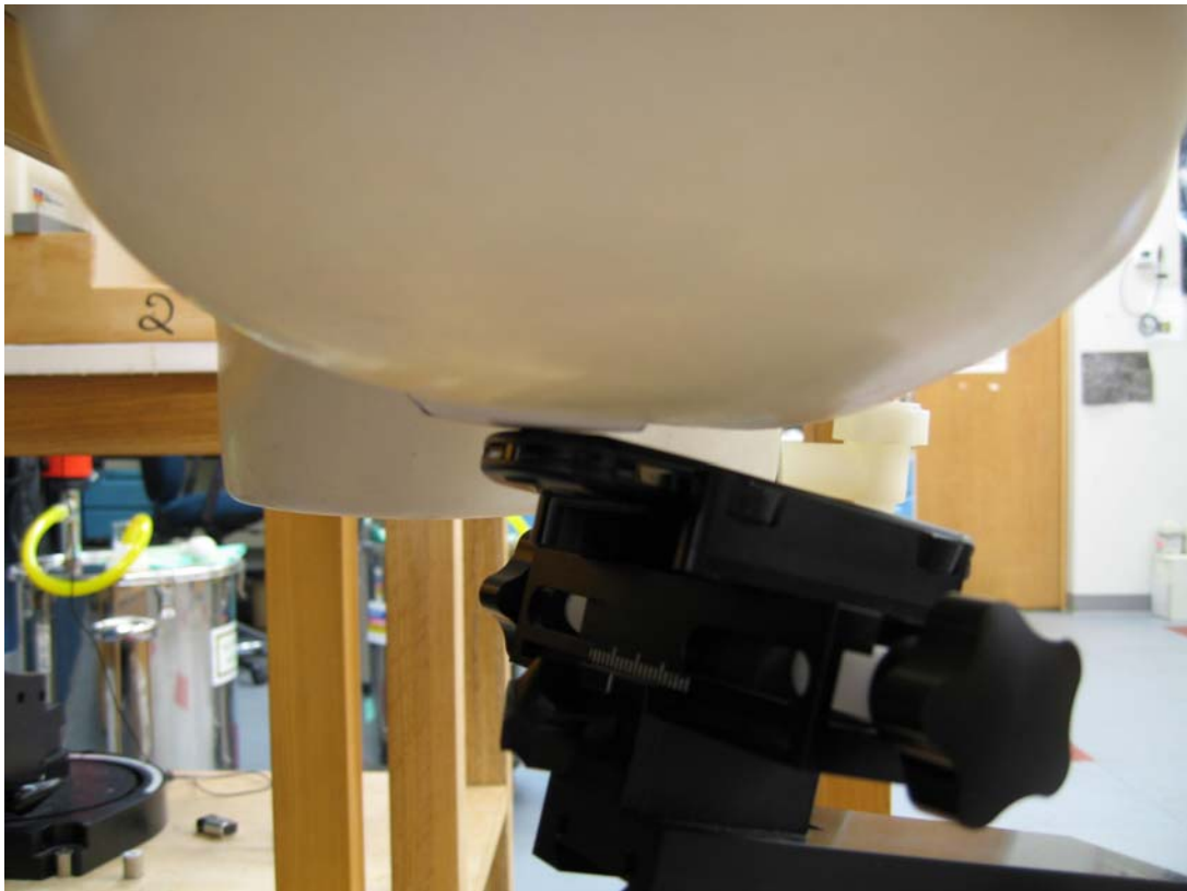
Figure 6 – Transceiver against head, 15° Tilt position
