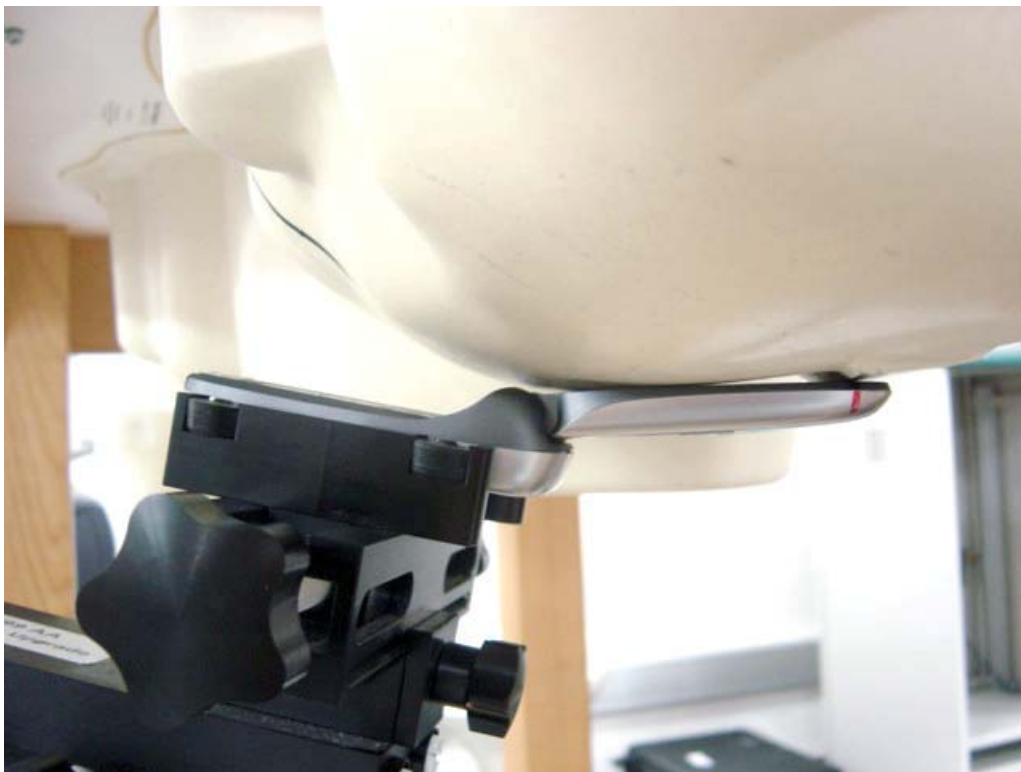
Figure 5. Phone Against the Head Phantom (Cheek Touch)
