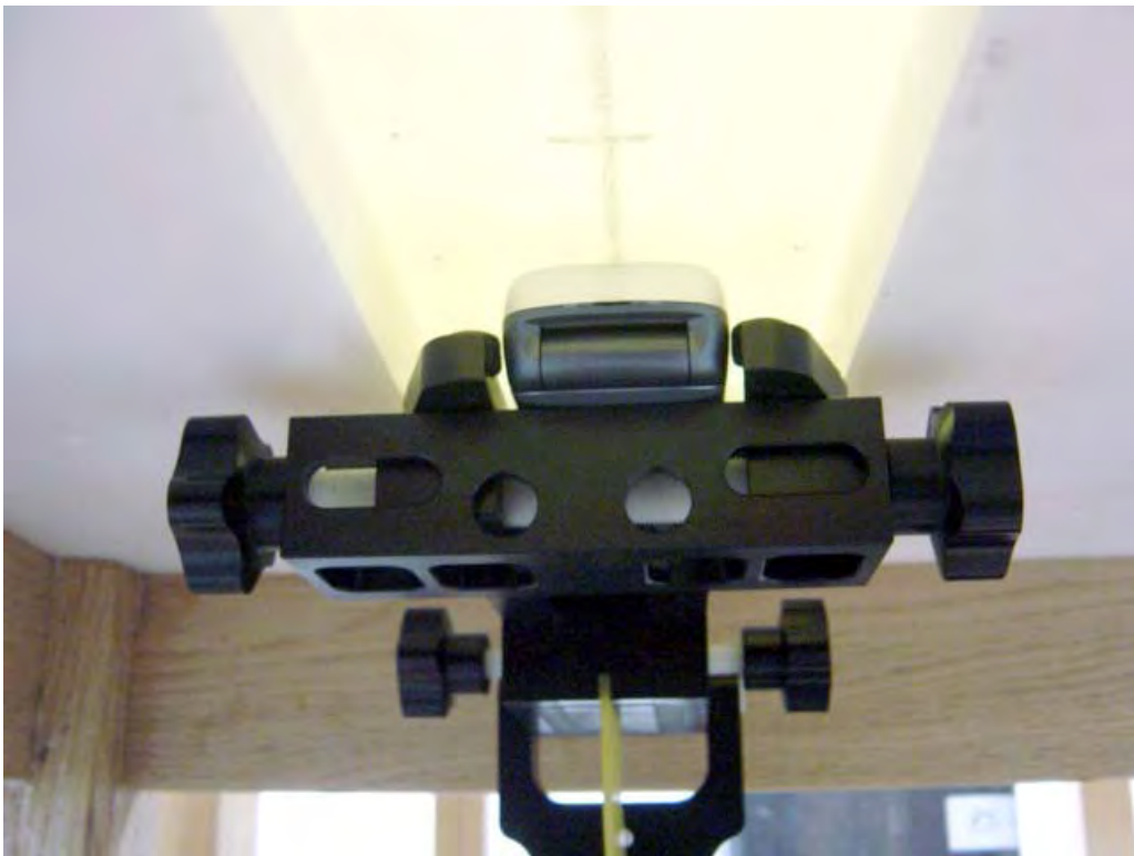
Figure 4. Phone Against the Flat Phantom
