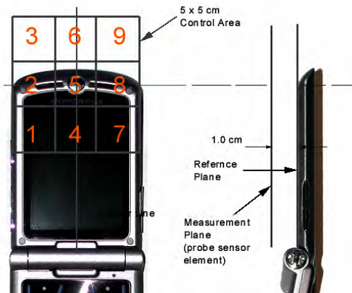
Figure 13 E/H-Field Emissions Test Setup Diagram
