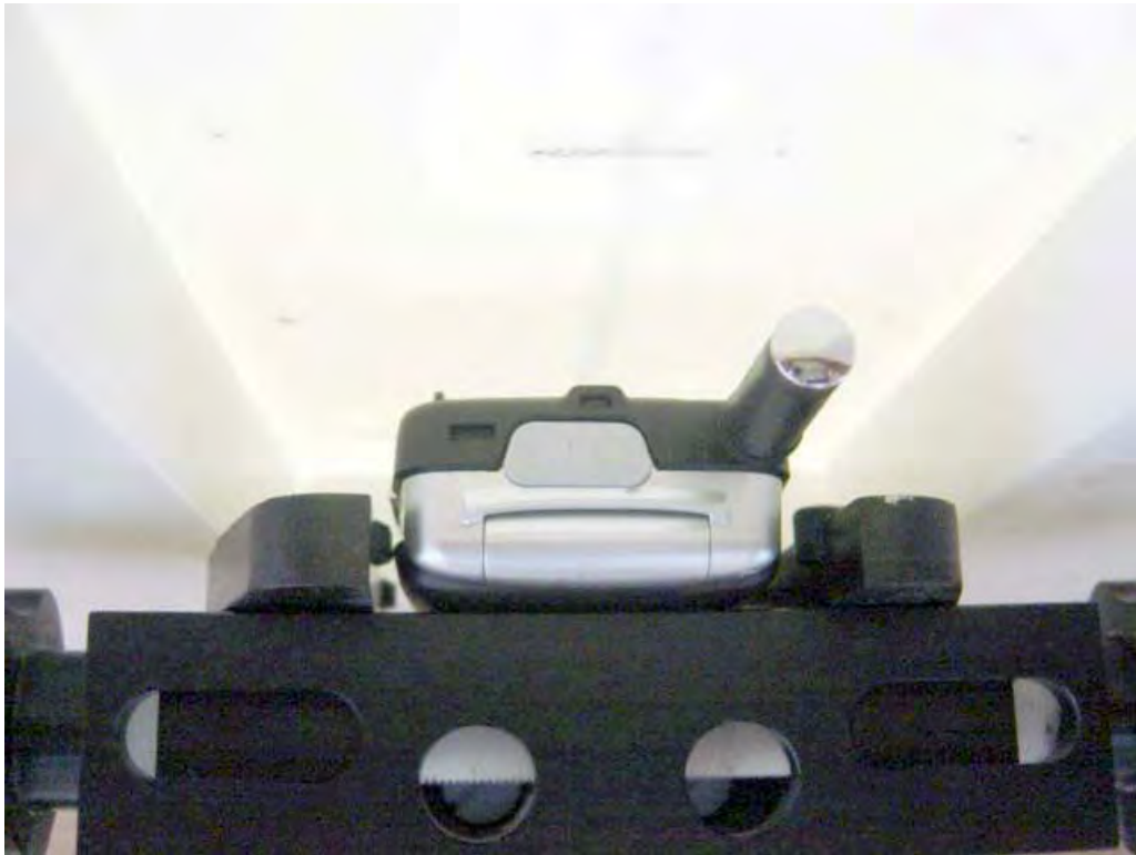
Figure 7. Phone Against the Flat Phantom; antenna retracted
