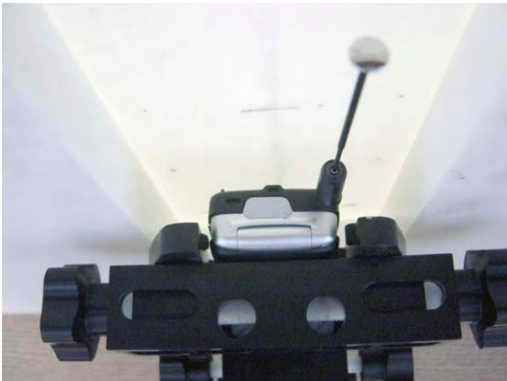
Figure 8. Phone Against the Flat Phantom; antenna extended
