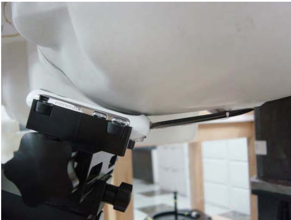
Figure 5. Phone Against the Head Phantom (Cheek Touch)
